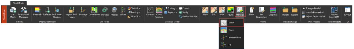
The **Manage » Mesh** option is used to generate fault meshes based on fault data from the design file. This option constructs a fault mesh around the existing **Corridor**, offsetting the fault line to its right and left side, and projecting it to the **Top** and **Bottom Elevation** or **Mesh**. To access this option, select **Faults » Manage » Mesh** from the **StratModel** ribbon.
