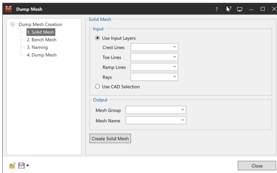
The **Dump Mesh** option allows users to create a dump mesh solid using spatial boundary definition, bench height, and block naming components. The following image is an example output of the **Dump Mesh** option.
