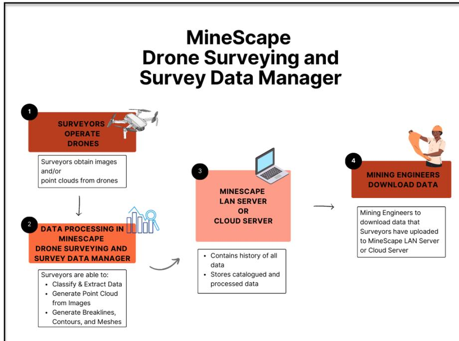
Through MineScape **Drone Surveying** Product, Surveyors can:
