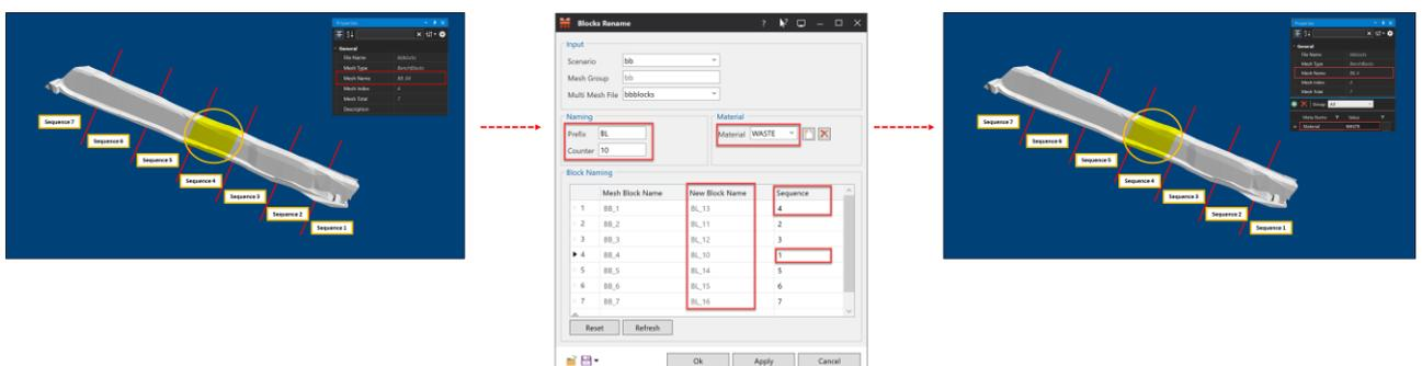
In the provided example, the solid mesh name changes from '**BB\_4**' to '**BL\_10**', and the mesh index shifts from the **4<sup>th</sup>** to the **1<sup>st</sup>**.
