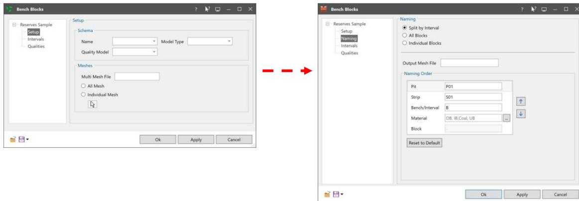
The **Naming** node can be used to construct the name for the solid mesh. The Naming Order will be displayed when the **All Blocks** or **Split Mesh Blocks by Interval** option is selected. The **Naming Order** has five (5) naming hierarchies: **Pit**, **Strip**, **Bench/Interval**, **Block**, and **Material**.
